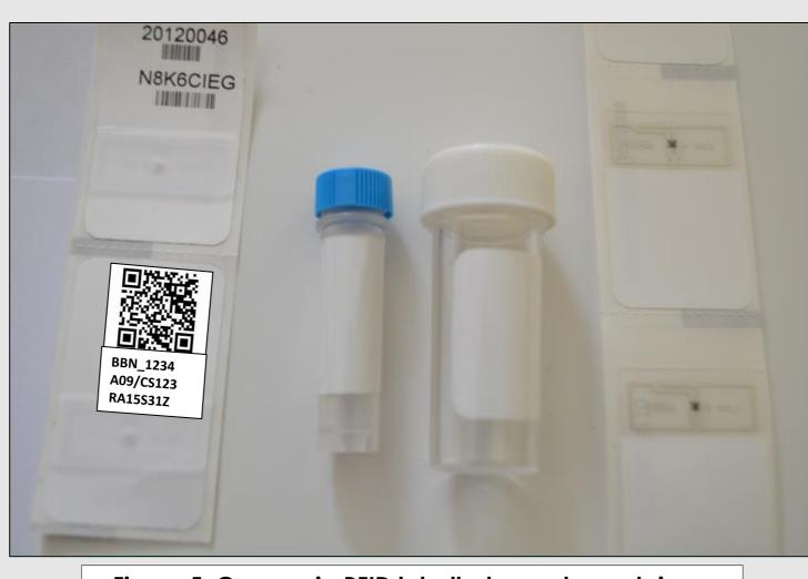
Figure 5: Cryogenic RFID labelled sample containers
