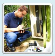
Once a sampler has reached each targeted sampling point, the process of taking samples can begin. The sampler will use a selection of equipment to ensure a representative sample is taken using the correct bottles and that a number of field measurements are taken.
