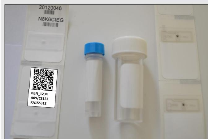
Figure 5: Cryogenic RFID labelled sample containers
