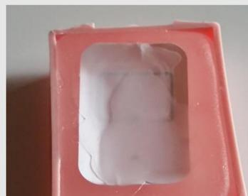
Figure 3: RFID label embedded in wax in cassette holder allows for easy sample tracking
